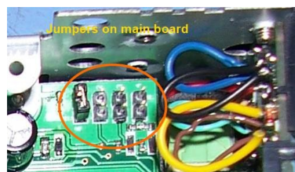
Jumpers on main board behind microphone socket
